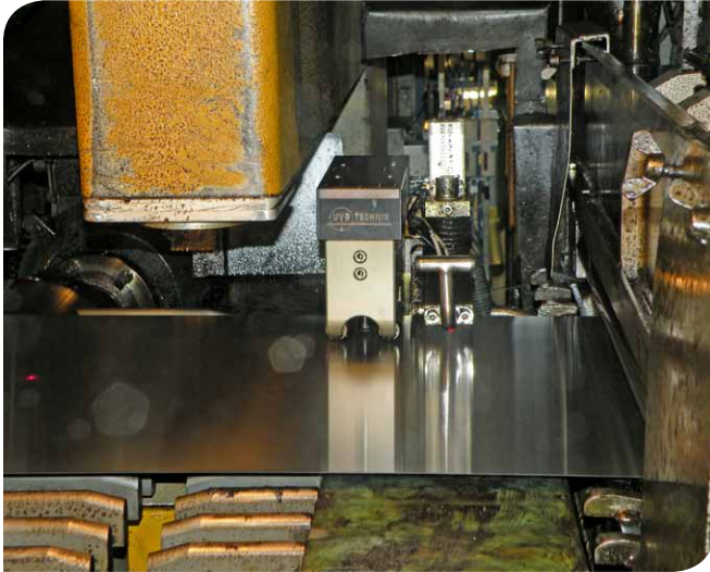
C.D. Waelzholz (werk Wickede), Germany, bimetal, cold rolling mill - Contact thickness gauge used for on-line calibration of X-ray gauge
