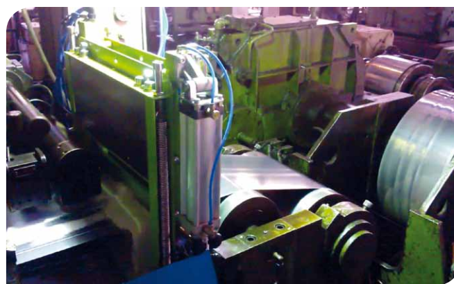
SUPERMAX, India, steel, reversing rolling mill
